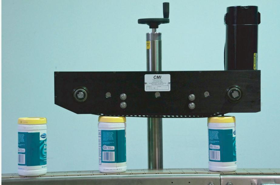
The Certified Machinery Cap Press unit is designed to bolt onto a customer's existing conveyor line and allows a cap to be pressed/applied into position on a mating component while in motion. It can also be used as a stabilizing device on tall or unstable products prior to other packaging operations.
