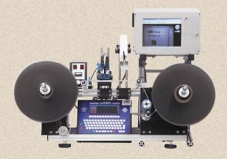
The LPVS integrates the Wolke m600 thermal inkjet printing system, printing serialized barcodes on a label transport system for track and trace requirements.
